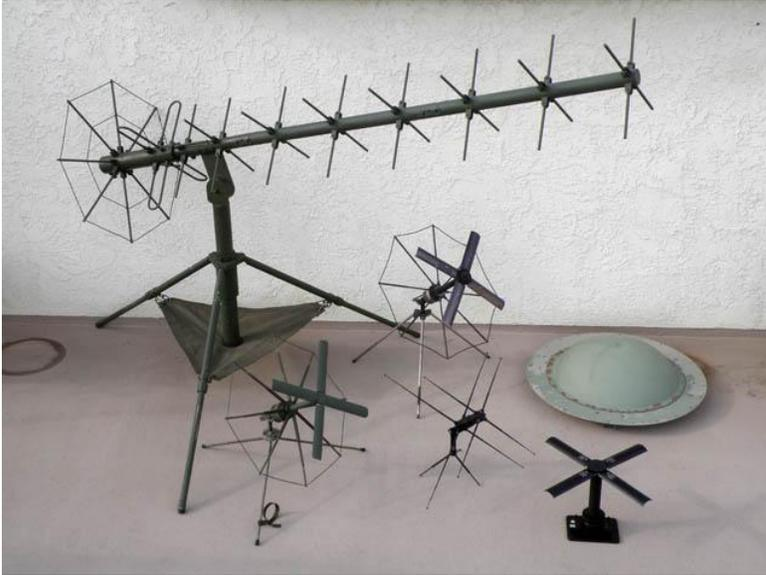
The large crossed Yagi to the far left has considerable gain over most models, which comes in handy when pointing low on the horizon and to better close the satellite link when other stations are using low power or smaller antennas. This particular model is a Dorne & Margolin DM C122 with a maximum gain of 14dBic. The “ic” references to a circular polarized isotropic antenna.
